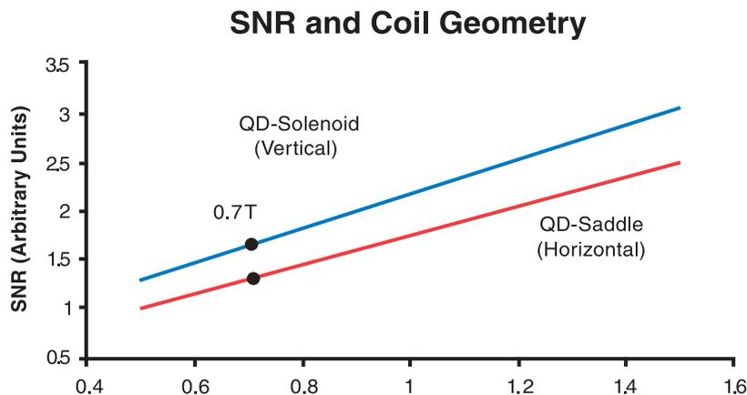
Note that for all field strengths, the QD-Solenoid combination coil SNR is 30% higher than that of the QD-Saddle type employed in a horizontal field application.
